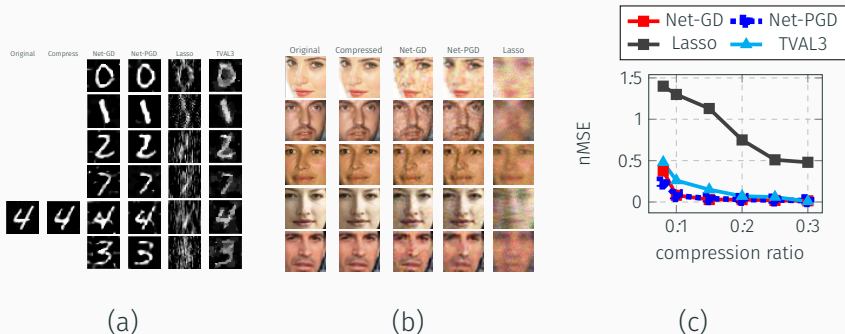
Figure 1: (CS) Reconstructed images from linear measurements (at compression rate = 0.1) with (a) = 78 measurements for examples from MNIST, (b) = 1228 measurements for examples from CelebA, and (c) nMSE at different compression rates = for MNIST.
